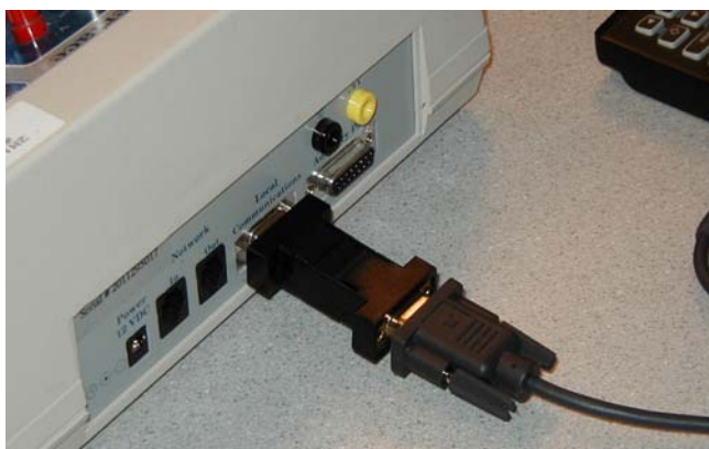
Figure 2. PDA serial cable attached to the LabWorks interface using a null modem gender changer.
